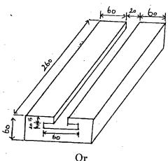
Calculate the machining time required to produce one piece of the (b) component shown in Fig. given below starting from f 25 mm bar. The following data is available.
